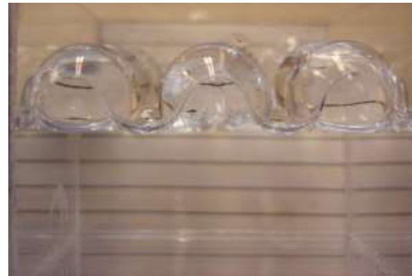
Fused silica spheres. Johnson & Johnson baby oil-Drakesol 260 oil mixture.
